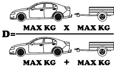
$$D = \frac{\text{MAX KG} \times \text{MAX KG}}{\text{MAX KG} + \text{MAX KG}} \times 0,00981 \leq 8 \text{ kN}$$
